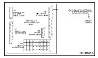
Figure 6-10 Low Fuel Switch (Level or Pressure)
